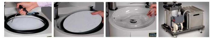
Retractable water hose for easy cleaning Simple exchange of working discs
