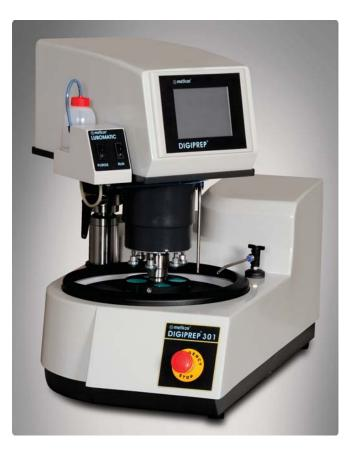
Upon completion of the cycle, an acoustic signal lets the operator know that the cycle is over and the samples are ready for the next step. When required, it is also possible to intervene in the program and change the parameters without stopping the instrument.
