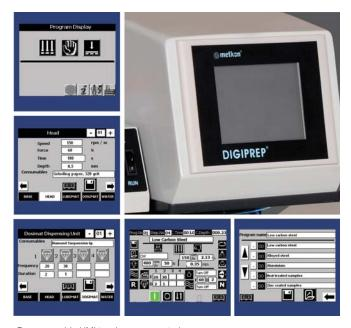
Programmable HMI touch screen controls
